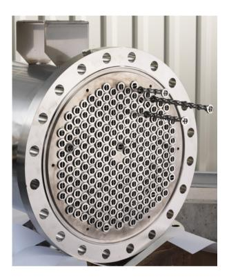
radial mixing effect significantly increases the heat transfer at the tube wall.
