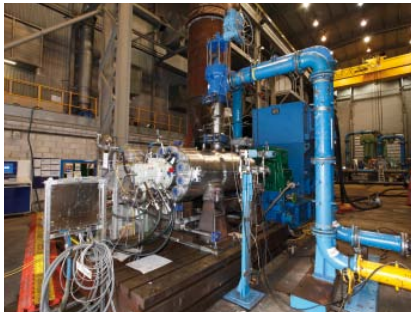
Bare pump undergoing performance testing
